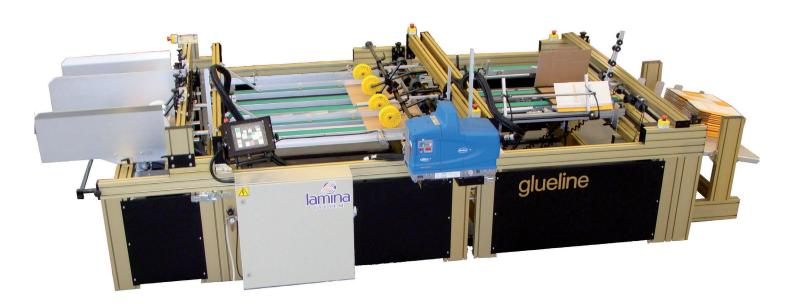
Lamina Glueline is a fully automatic non-stop gluing and folding machine for one piece or two piece boxes. The machine works with two heavy duty vacuum controlled belt feeders which feed in the one or two pieces. By using Laminas registration system and non-stop feeder, the machine is extremely effective for two piece boxes.
